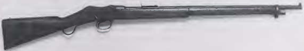
Figure 19 The Unofficial Conversion Martini-Enfield Mark I, W.A. Pattern. There is evidence that William Vernon Needham, a local gunsmith and Armourer to the Forces, did the conversions. This specimen, in poor condition, no longer has its original Metford profile barrel. (Photo D. Elford).
